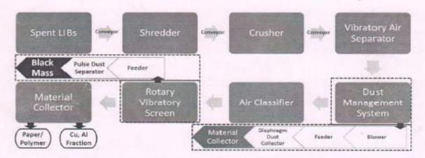
Fig.1: Tentative Illustration of Proposed Battery Dismantling and Powder Separation Setup
